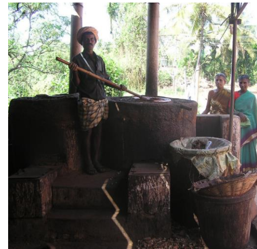
FUEL-EFFICIENT ARECANUT BOILER (TIDE Technologies)
